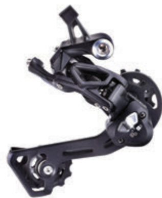
MicroShift XCD11 with clutch
