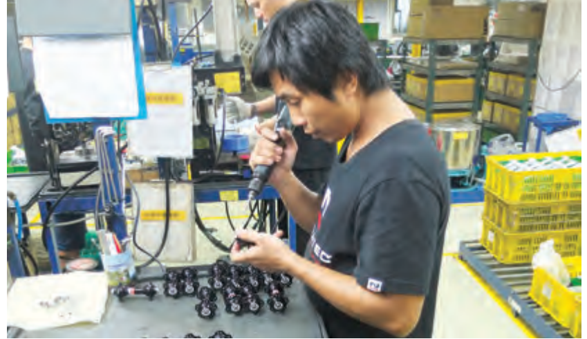
Experienced workers assemble Novatec hubs.
