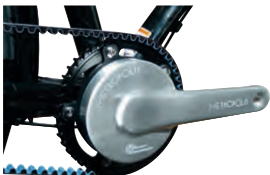
The FSA Metropolis 2-gear system, adapted for a belt drive
