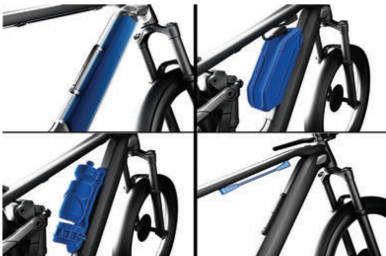
Shimano's dual battery system as used on the Focus Jam and Bold e-MTBs.
