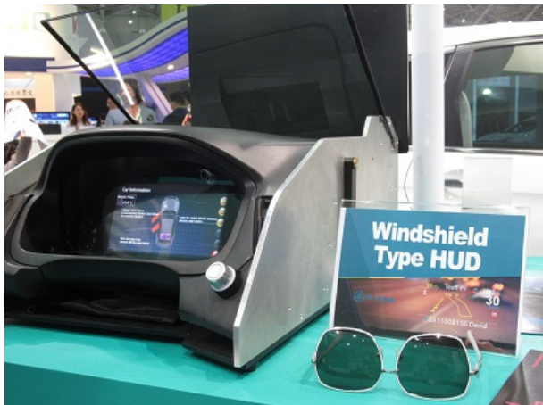
Windshield-Type HUD. It's made visible for drivers with sunglasses on. (photo: EE Times)
