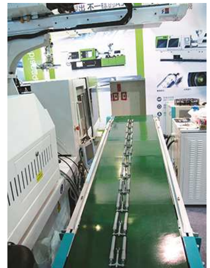
An FE machine produces metal medical parts using a mixture of steel and plastic powders.
